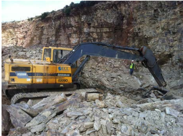
iii). An Akerman 3060° slew with plain bucket which was recorded at 84 dB L_{Aeq} at 10m,
