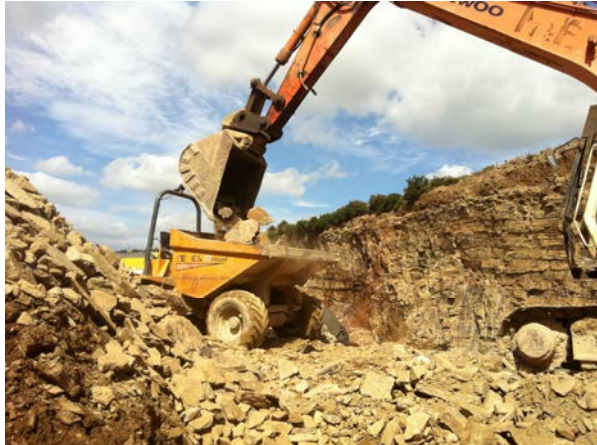
iii). An Akerman 3060° slew with plain bucket which was recorded at 84 dB L_{Aeq} at 10m,
