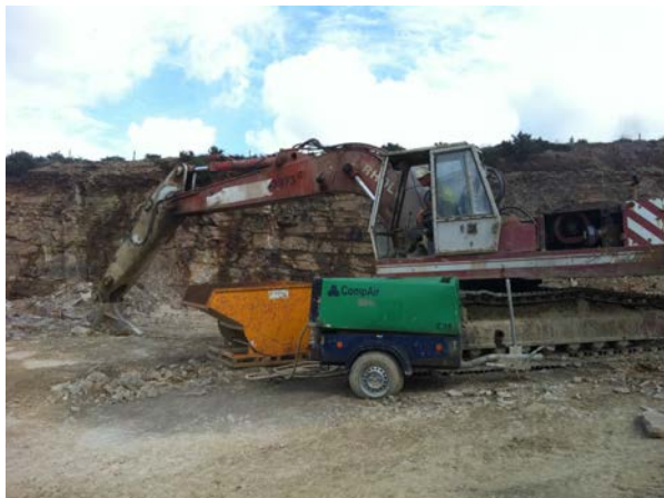
iv). An ONK slew with “ripper” which was recorded at 85 dB L_{Aeq} at 10m;
